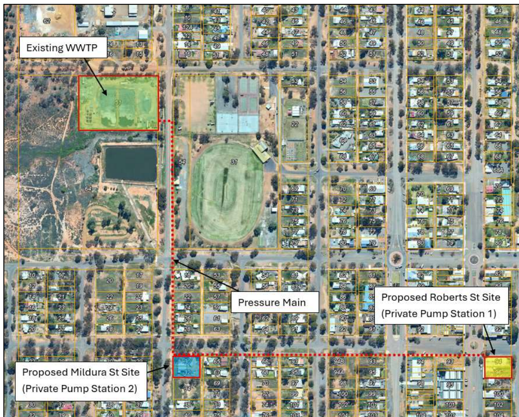
Figure 2: Proposed Sewer Servicing
