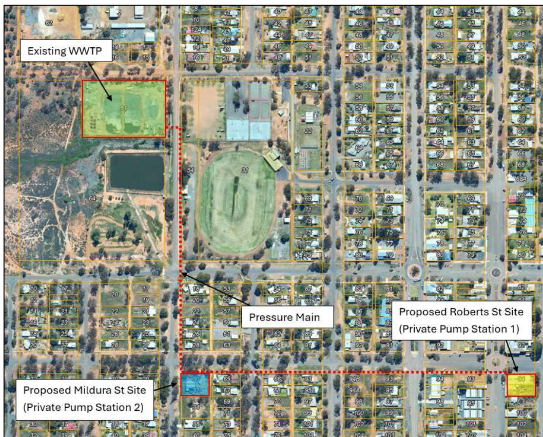
Figure 3: Expected Sewer Servicing
